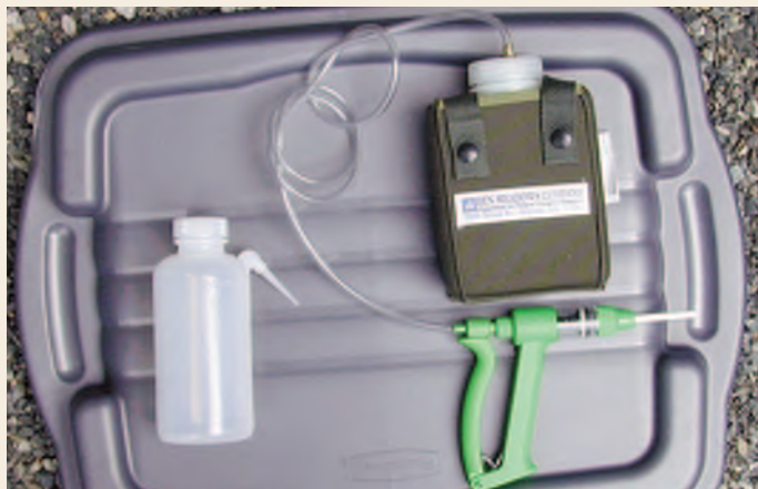
Hollow stem injection tools.
